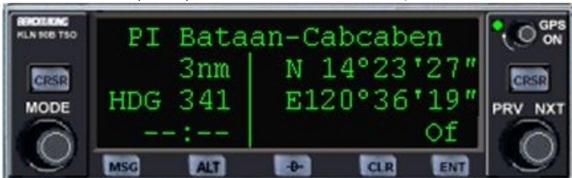
Clicking on the "PRV-NXT" button moves you up and down in the GPS Program Leg list. In this case, clicking on the "NXT" side of the button moves us from Bataan-Cabcaben to
