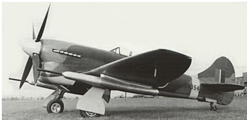
A Vickers 47 mm "P" gun was tested on a Tempest V (SN354) just after the war. The large cannons were faired into slim, streamlined pods and carried on the bomb racks. The tests revealed that the weapon had potential, but no production was undertaken.
