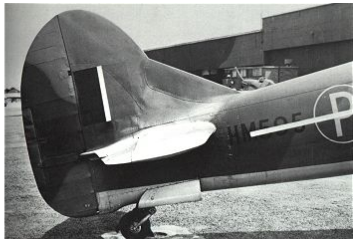
The first Tempest V prototype HM595, with the first stage of modification of the fin to improve directional stability.
